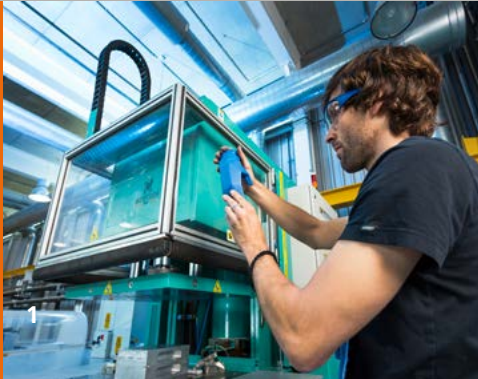
1 Wax injection molding.
